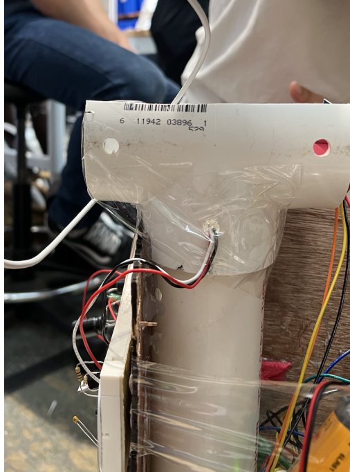
Figure 15: Side view of wires connected to switch threaded through hole in the PVC to attach to the electronics breadboard
