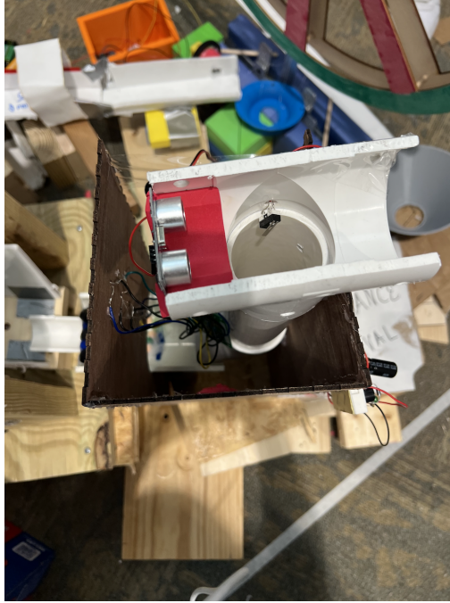
Figure 17: Top view of drop tower showing switch and ultrasonic sensor
