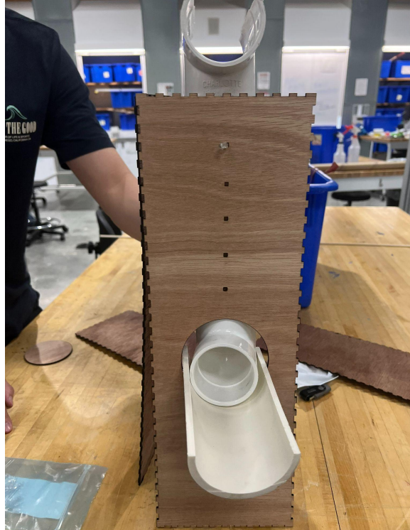
Figure 10: Front view of drop tower with holes for LEDs and exit ramp
